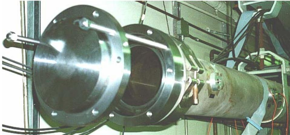
6-in shock tube and plate fracture test
